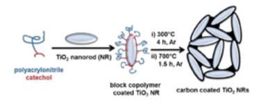
Fig.: Carbon coating approach of TiO<sub>2</sub> nanorods using anchoring block copolymer carbon precursor.
