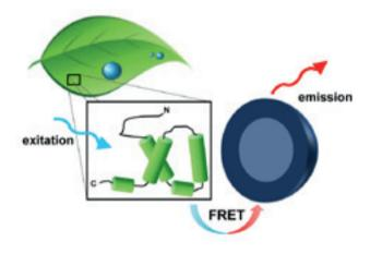
Fig.: LHC attached to the surface of a QD efficiently transfers its excitation energy to the inorganic nanocrystal.
