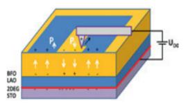
Fig.: Charge carriers are introduced locally into the electron gas at the interface by changing the ferroelectric polarization with a piezo force microscope.
