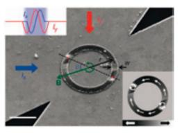
Fig.: Magnetization of a nanostructured permalloy ring.
